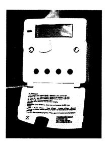
The timeclock is utilised to set the desired heating times while the 3 port control valve works constantly to attain and maintain the set temperature.
